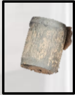
Hot Vertical Upsetting (Heading)
